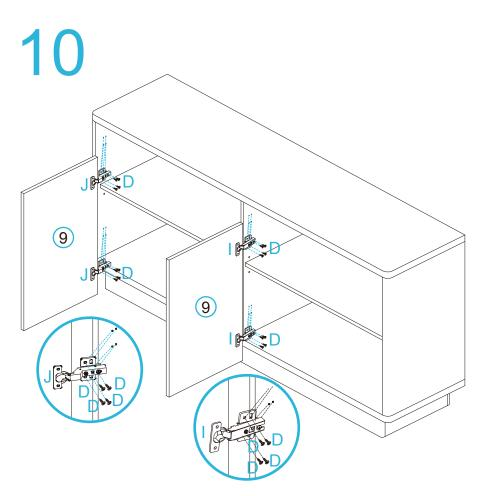
Attach 4 x hinge (J) and 4 x hinge (I) to panels [9] as shown and secure with 16 x screws (D). Tighten with a screwdriver.
